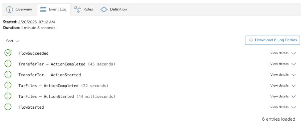
Figure 8.2: The Globus Flows UI showing the event log of the Tar and Transfer flow. Each task can be inspected to review outputs or debug failures. The flow access control roles and definition are available in other tabs.
