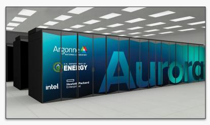
10K Nodes / 1M Cores / 60K GPUs 20 PB Memory / 230 PB Storage
